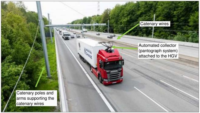
Figure i: Photograph of a Scania HGV operating on a catenary lorry 'eHighway' demonstrator in Germany, from Siemens (2020).
